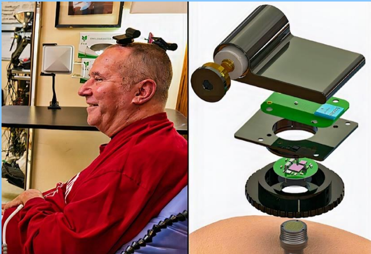
A participant in a clinical trial uses wireless transmitters that replace the cables normally used to transmit signals from sensors inside the brain. Source: BrainGate
